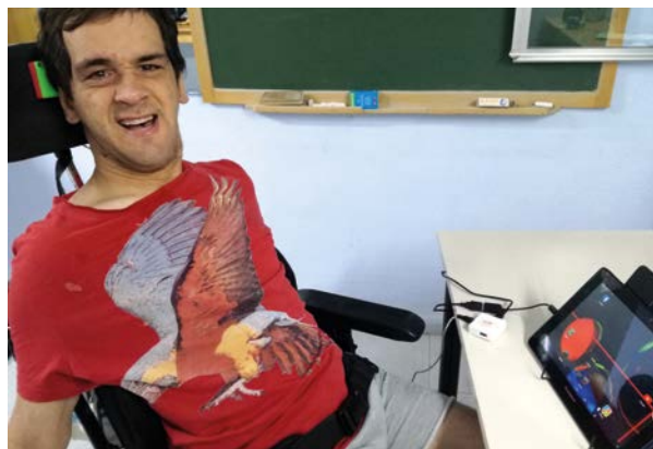
Mouse4all uses horizontal and vertical cursors as well as symbols and pictograms for input.
