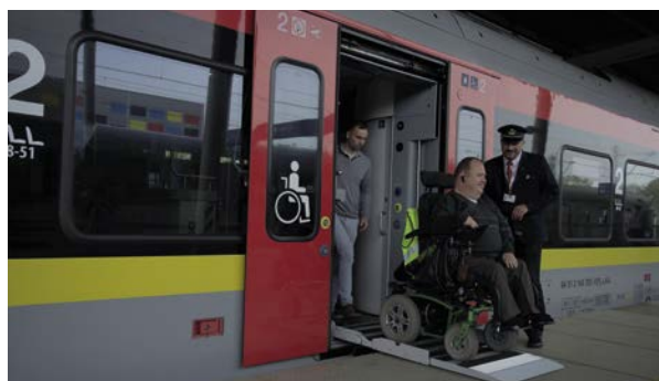
Facilitating individual mobility: This ramp enables people in wheelchairs to get off the train without any barrier.
